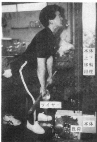
Fig.2 Pull movement in weightlifting competition (right) and measurement of mechanical power during simulated pull movement in weightlifting using Power Processor (left).
